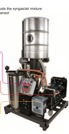
Hopper: Stainless steel hopper holds up to 10 hours of fuel.
