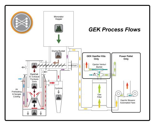
The GEK Gasifier Kits and the Power Pallet have different gas drive systems as shown in the GEK Process Flow diagram above. For the GEK Kits, the gas enters the gas filter, and passes through the ejector gas drive system. Here the air is then mixed for the flare.
