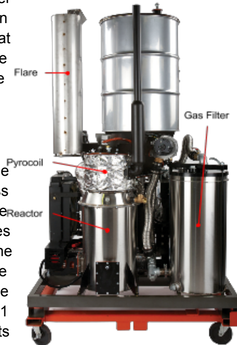
Reactor side of the Power Pallet
