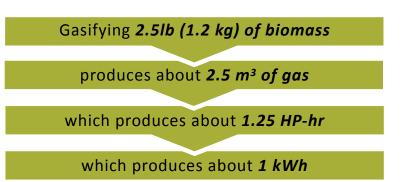
The best fuel for the GEK gasifier is chunky, dry, carbon-dense woody biomass. Fuels such as wood chips, wood chunks, nut shells, and coconut shells ranging in size from 0.5" to 1.5" (10mm to 50mm) are ideal.
