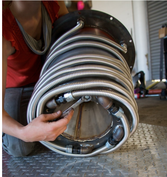
Figure 4: A view of the internal parts of the reactor. The air lines that pre-heat intake air using heat recovered from fresh wood gas.
