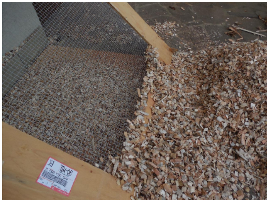
Sifting with the ½" screen to remove undersized pieces and fines. These fall through the screen.
