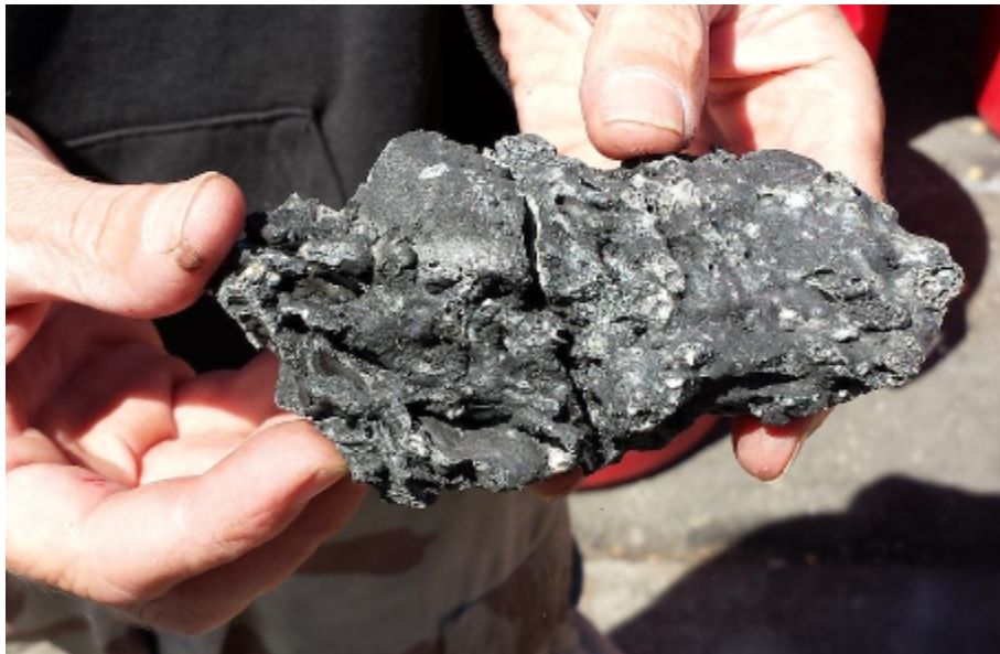
An example of one of the clinkers that fouled a reactor running a test on almond husks.
