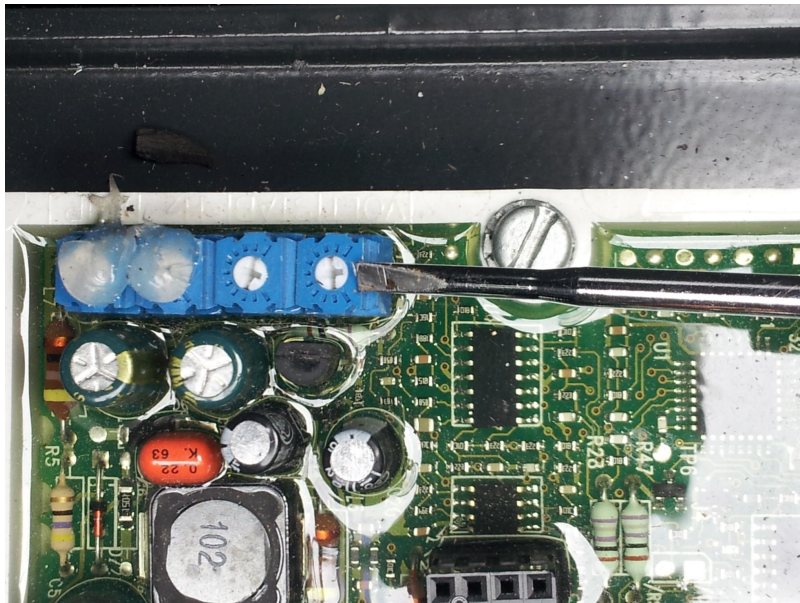
Location of the VOLT potentiometer
