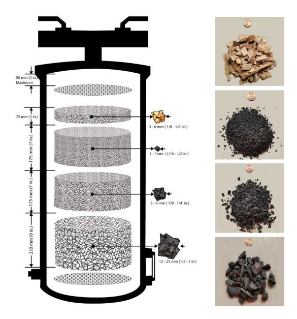
Depending on type and moisture of feedstock, the life of the filter can vary widely. If *Pfilt* reading is over 300 during operation on load, filter may need to be repacked. Inspect the top layer of the filter periodically, and if it is very dark, wet, or fouled by tar, repack the filter with new charcoal.
