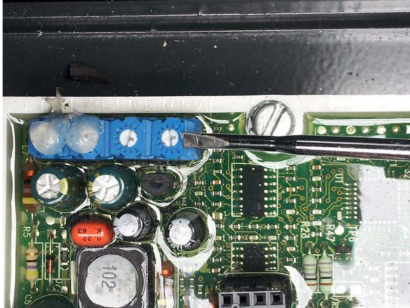
Location of the VOLT potentiometer
