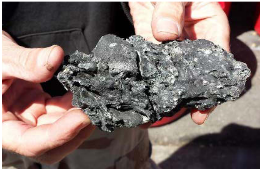
An example of one of the clinkers that fouled a reactor running a test on almond husks.
