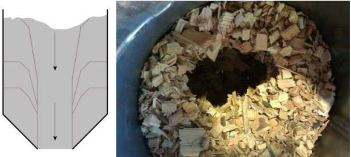
An example of rat-holing in feedstock.
