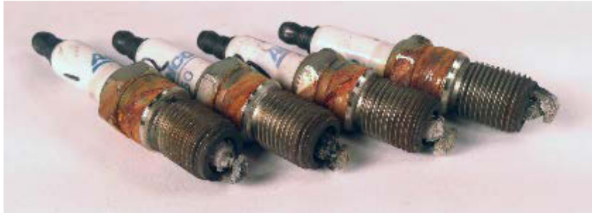
Examples of fouled spark plugs that caused malfunction.
