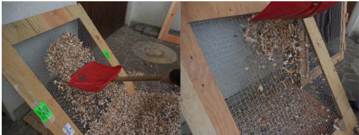
Sifting with the 1" screen to remove over-sized pieces. Over-sized pieces remain above the screen.
